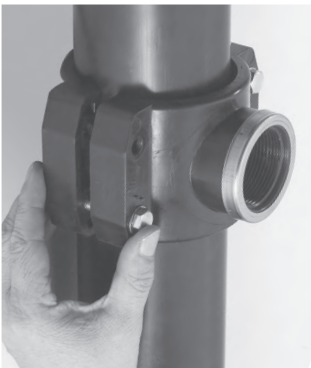
2. Taking care to seat gasket in the branch outlet, bolt both halves together.
