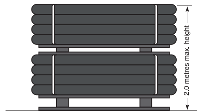
Storage of coils
